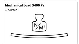
\*Due to glass-glass Multisol® Vitro laminate 50 % more load compared to standard Multisol® Integra
