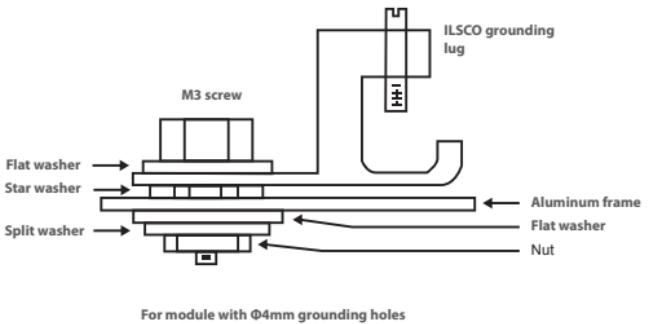
For module with Ø4mm grounding holes
