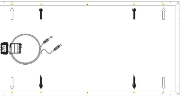
↑ Mounting holes for normal installation
